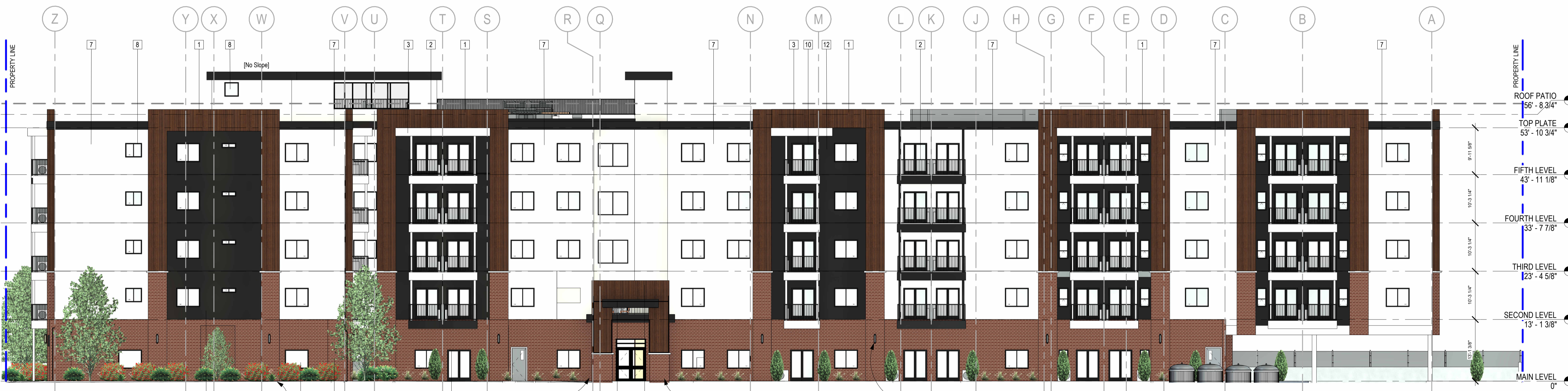
2 NORTH ELEVATION A3.00 3/32" = 1'-0"
