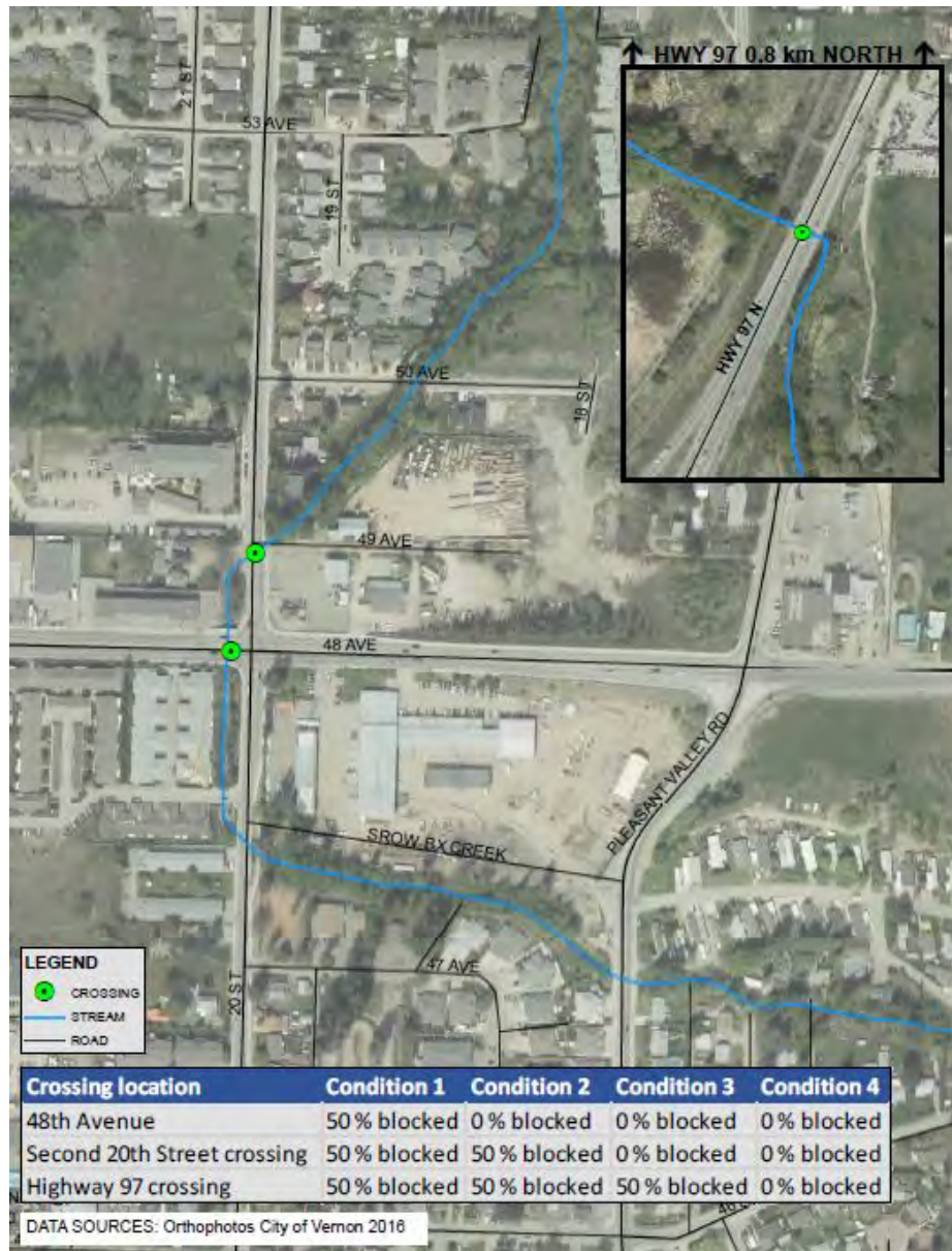
Figure 5.3 Modeled culvert sediment infilling locations.
