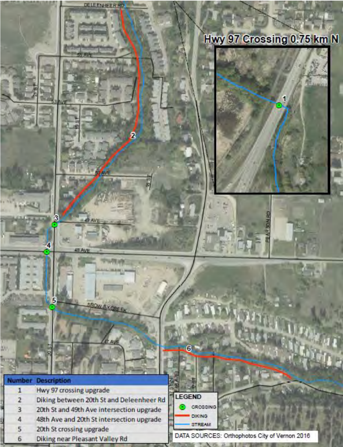
Figure 8.1 Suggested structural mitigation options for Upper B.X. Creek.
