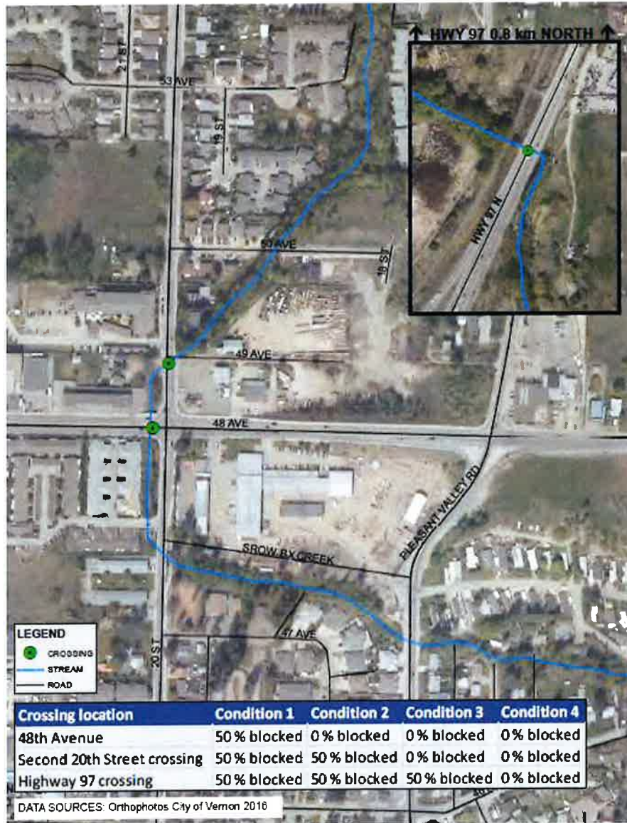
Figure 5.3 Modeled culvert sediment infilling locations.
