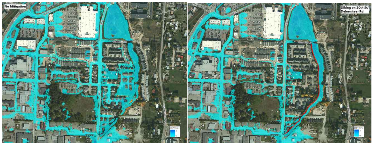
Figure 7 - unmitigated flooding during design event along Upper BX Creek, mitigated (right)
