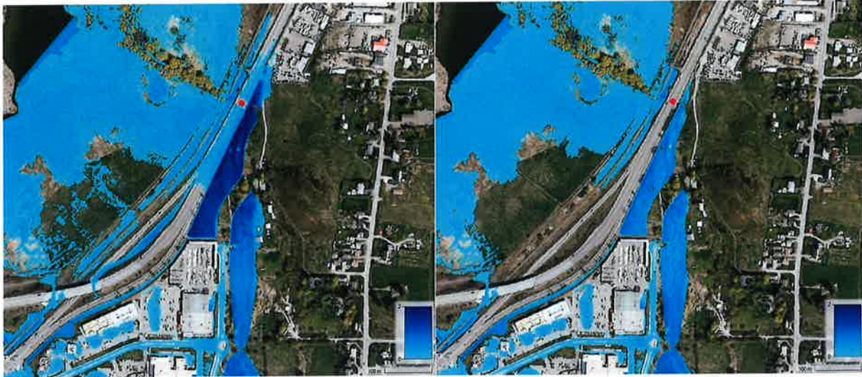
Figure 2.7 Flood extents at Hwy 97 under current conditions (left), with proposed upgrade (right) based on model results for the design flood event. Blue gradient indicates depth of water in meters.
