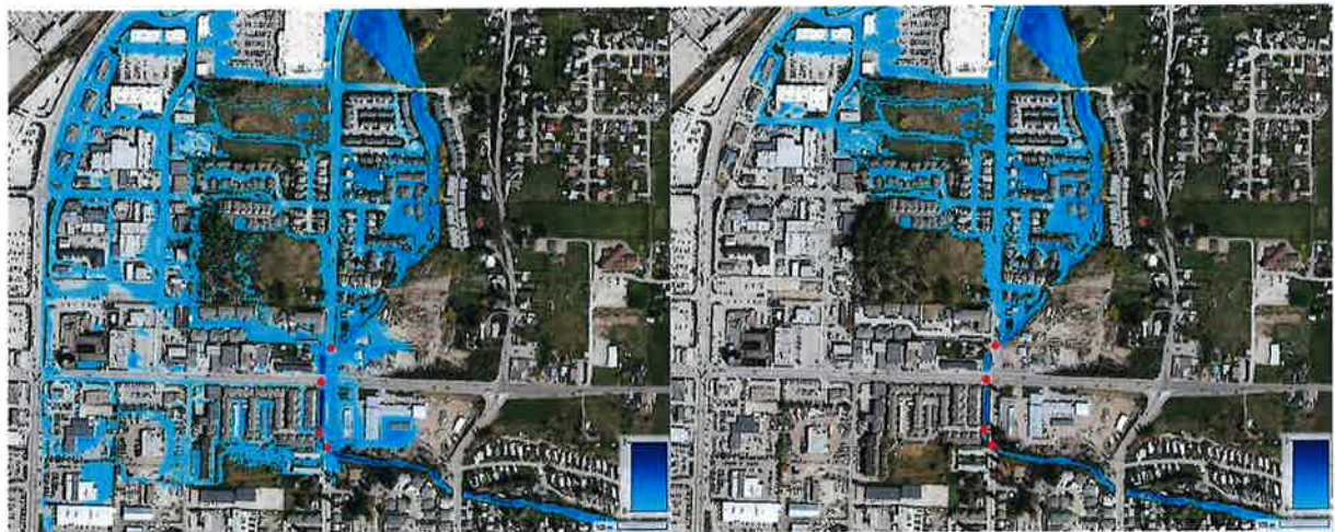
Figure 2.3 Flood extents at 20th Street crossings under current (left) and mitigated (right) conditions based on model results for the design flood event. Blue gradient indicates depth of water in meters.
