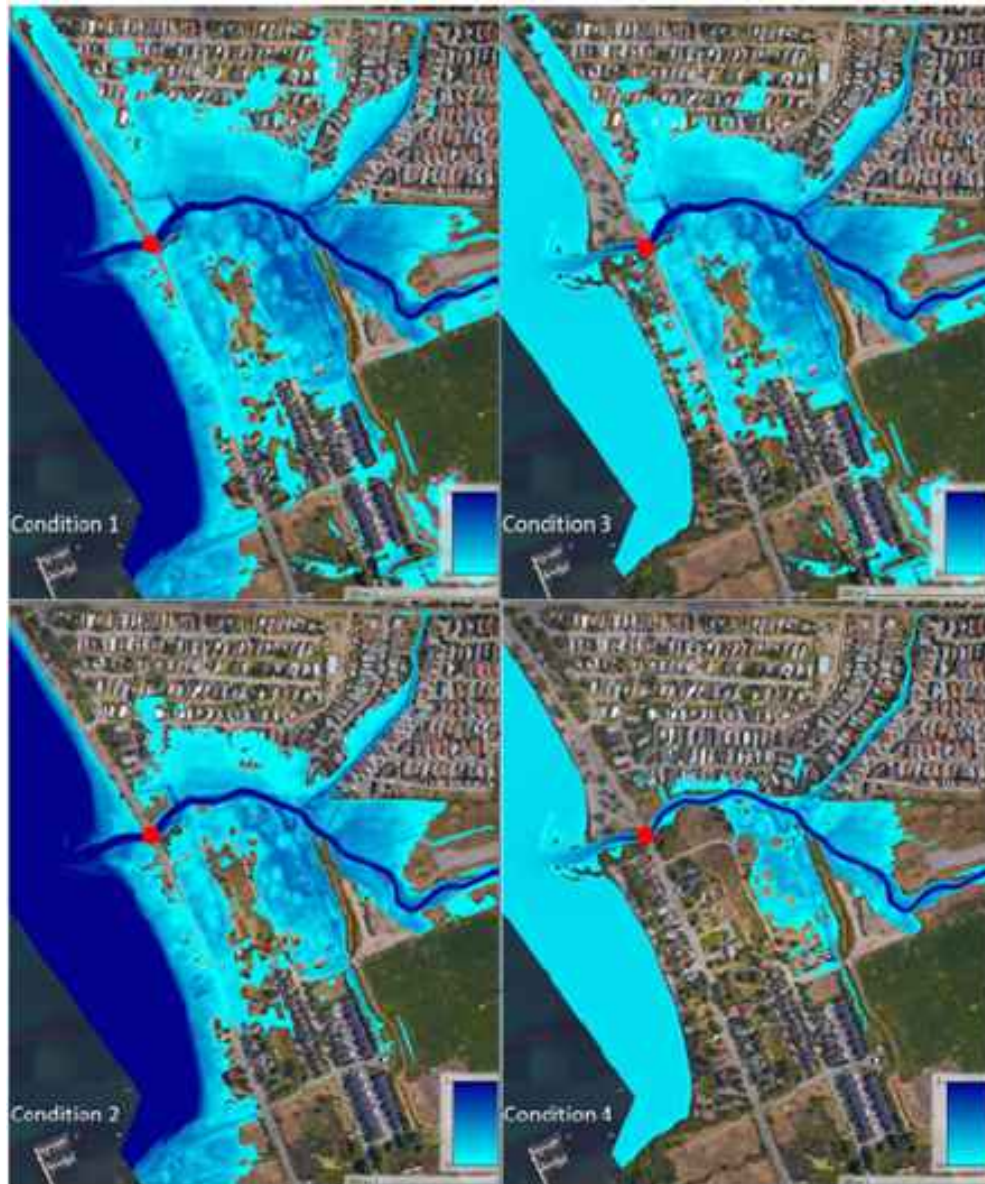
Figure 10 – Flooding scenarios at Lakeshore Road creek crossing
