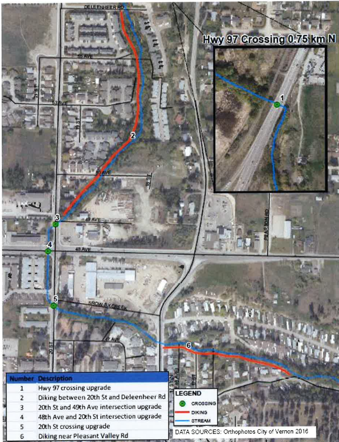
Figure 2.1. Suggested structural mitigation options for Upper B.X. Creek.
