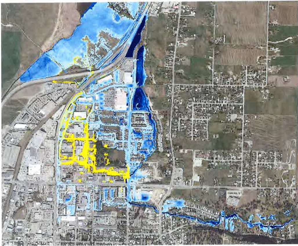
Figure 5.4 Comparison of flood extents for culvert infilling Condition 2 (yellow + blue) and Condition 3 (blue) for the design flood.
