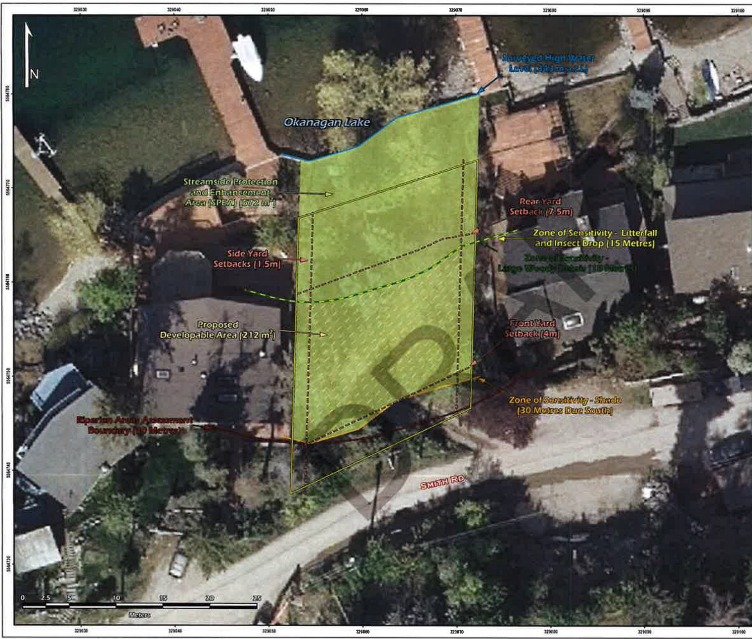
FIGURE 2 Riparian Areas Protection Regulation Project: Environmental Assessment Location: City of Vernon Project No.: 20-3617 Prepared for: CDG Enterprises Prepared by: Ecoscape Environmental Consultants Ltd. Dan Austin, GIS Specialist Coordinate System: NAD83-UTM Zone 11 Imagery: ESRI World Imagery Field Visit: N/A Map Date: January 18, 2022
