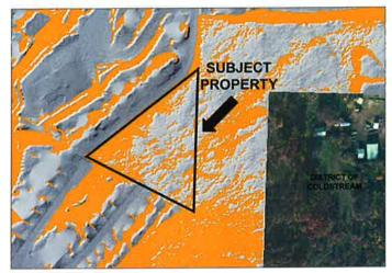
Figure 3: LIDAR with ≥30% Slopes
