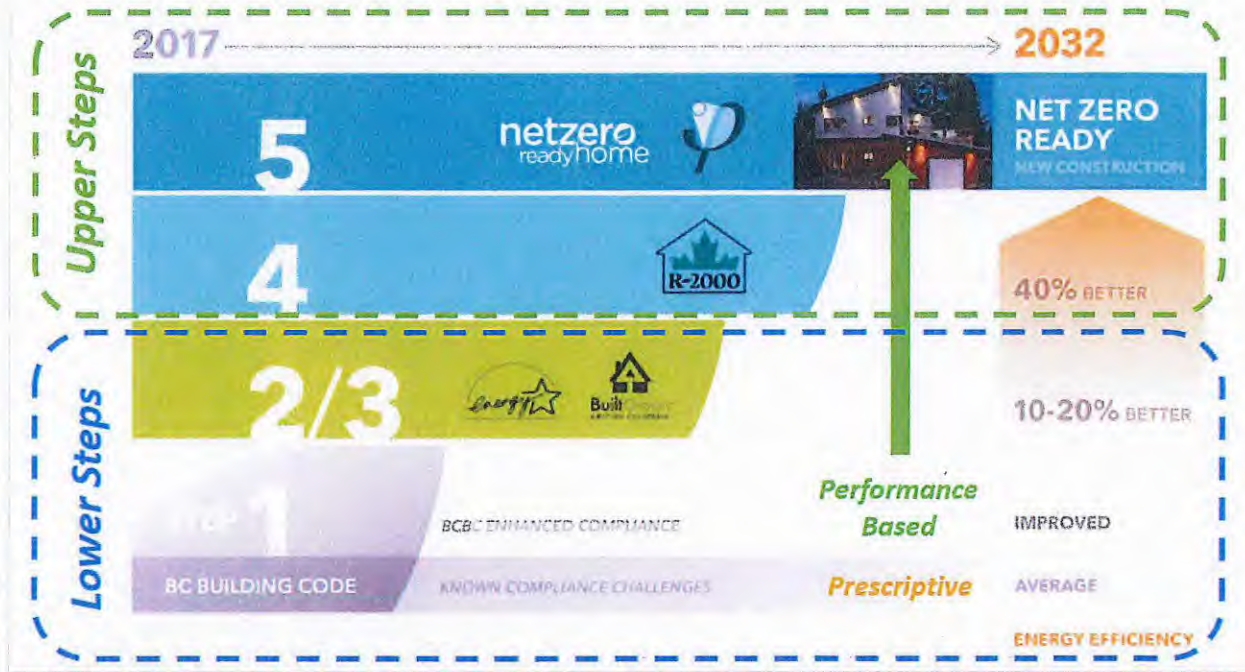
Figure 1. BC Energy Step Code: Steps for Part 9 Buildings
