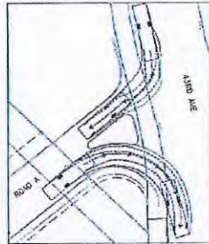
TURNING DETAIL 2 ROAD A - ROAD B INTERSECTION
