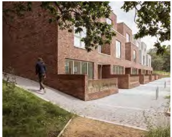
Figure 39: Ensure access ramps, exterior lifts, and related elements are visually integrated with the building design and site plan to avoid a disjointed appearance.
