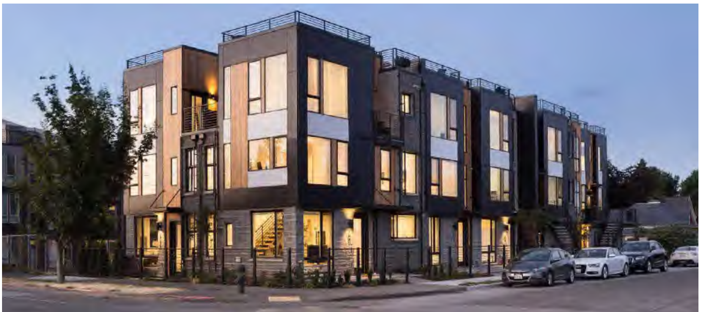
Figure 6: On corner lots, design buildings to face and activate both streets, with consistent facade treatment and entrances that engage each frontage.
