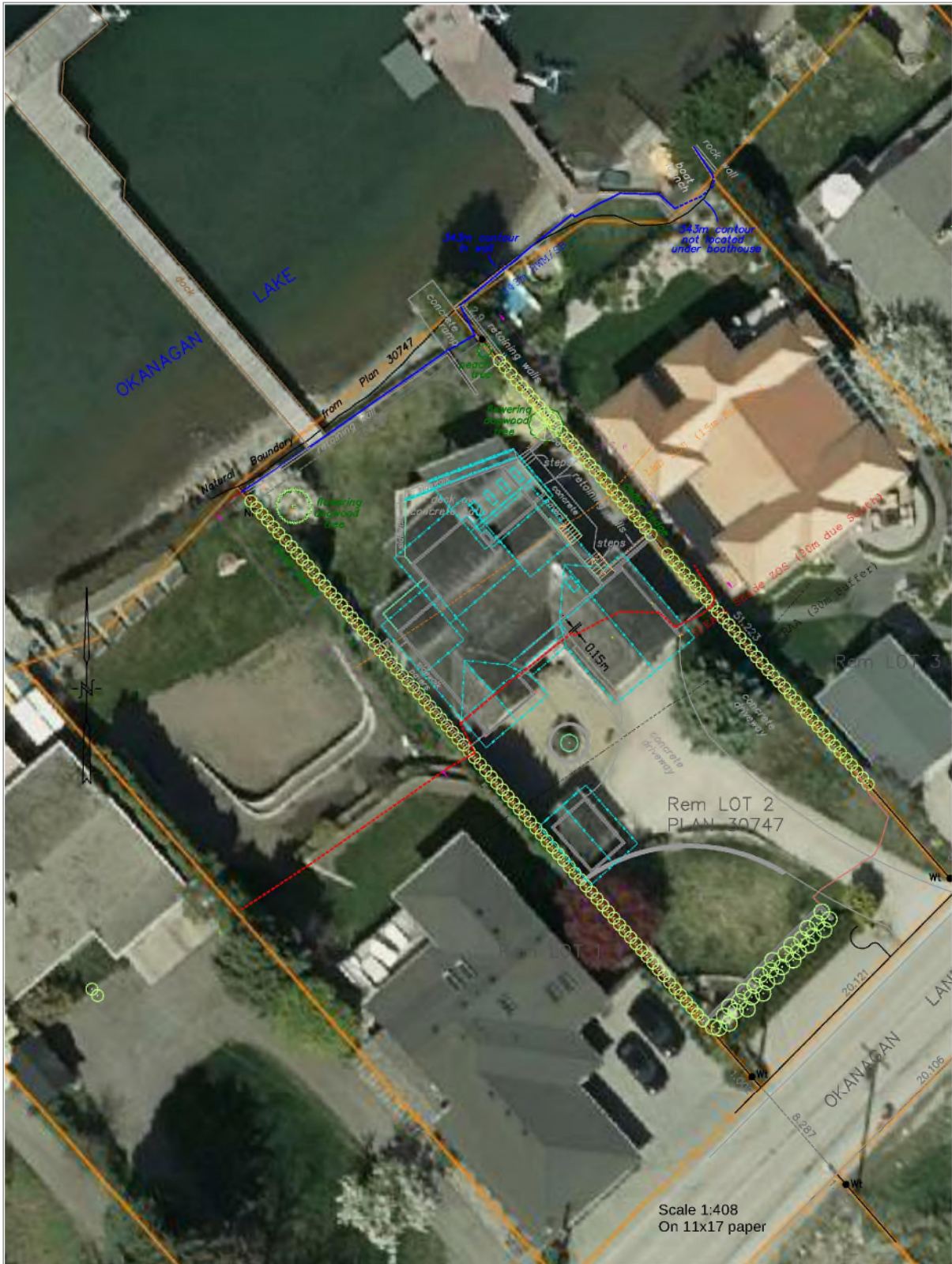
Figure 1A: Site plan with existing structures (grey), existing roof-line (light blue), existing trees and hedge, aerial image and RAPR determined SPEA (red dashed).
